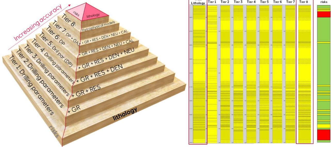
Figure text: The 8 steps (tiers) and input data for the REAL technology presented next to the true lithology and automatic trip risks.
