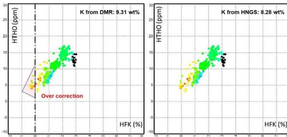
Figure 1 Potassium correction comparison between DMR and HNGS reading in a TBO borehole. The X axis represent the K content from HNGS, the Y axis the Th content from HNGS.
