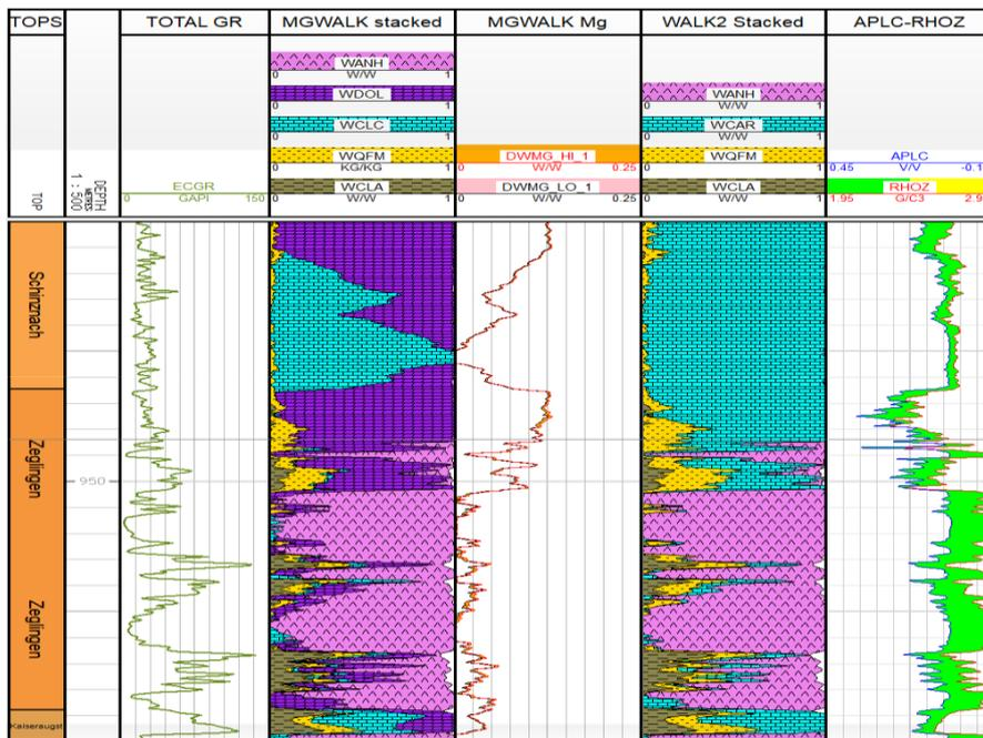
Figure 2 Comparison of standard ECS processing (WALK2) with advanced ECS acquisition and processing (MGWALK)
