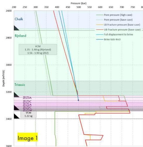
Thin anhydrite → shoe placement not possible. Still potential for overpressure.
